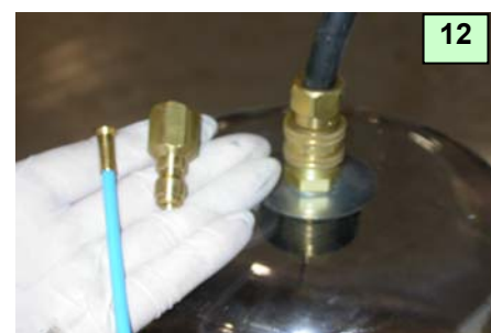
12: Take the Plastic Liner and the male Conduit Connector from Payoff Kit # K2860-1
