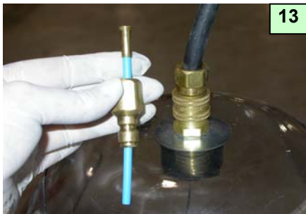
13: Put the Plastic Liner into the male Conduit Connector
