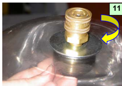
11: Take the Conduit Connector (female) from Payoff Kit # K2860-1 and assemble it according to the picture.
