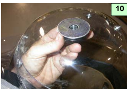
10: Take the Washer from Payoff Kit # K2860-1 and place the Washer on top of Payoff Cover
