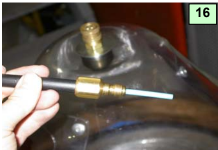
16: Conduit is now assemble with the male Conduit Connector and the Plastic Liner
