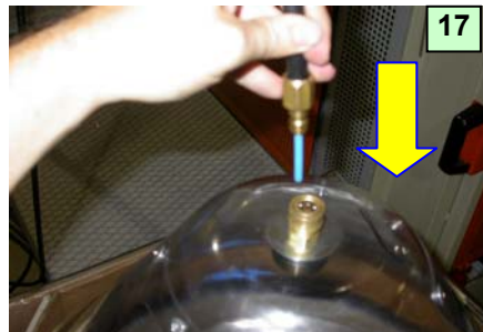
17: Assemble male and female Conduit connectors
