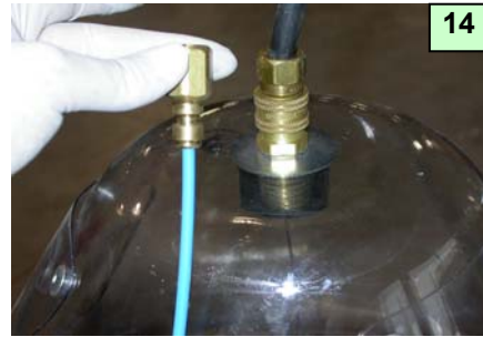
14: Plastic Liner inside the male Conduit Connector
