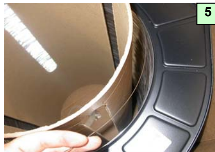
5: Pull the wire inside the plastic ring
