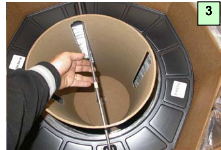
3: Remove the steel bar
